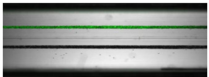
**Figure 1. Effect of low- and high-density particles on levitation height.** The particles shown in green are fluorescently labeled particles of a low-density polymer, and consequently levitate high in the separation channel. The non-labeled (black) particles consist of a different, higher density polymer and as a result levitate lower in the channel.
