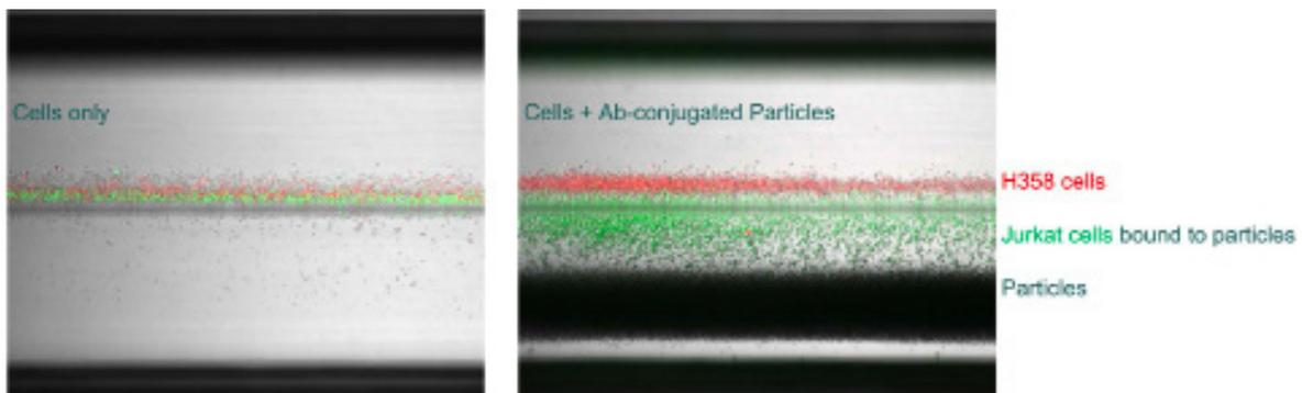
**Figure 2. Separation of cell types with density particles.** In the first two images on the left, the fluorescently labeled Jurkat cells (green) are located at the bottom of the channel due to the highest concentrations of magnetic particles. As the concentration is decreased, the Jurkat cells can be observed levitating at increased heights. In the final image on the right, there are no magnetic particles present, resulting in no differences in levitation height between the two cell types.
